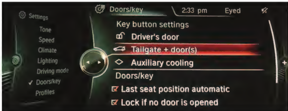
5 Series LCI configuration of third button in central information display
